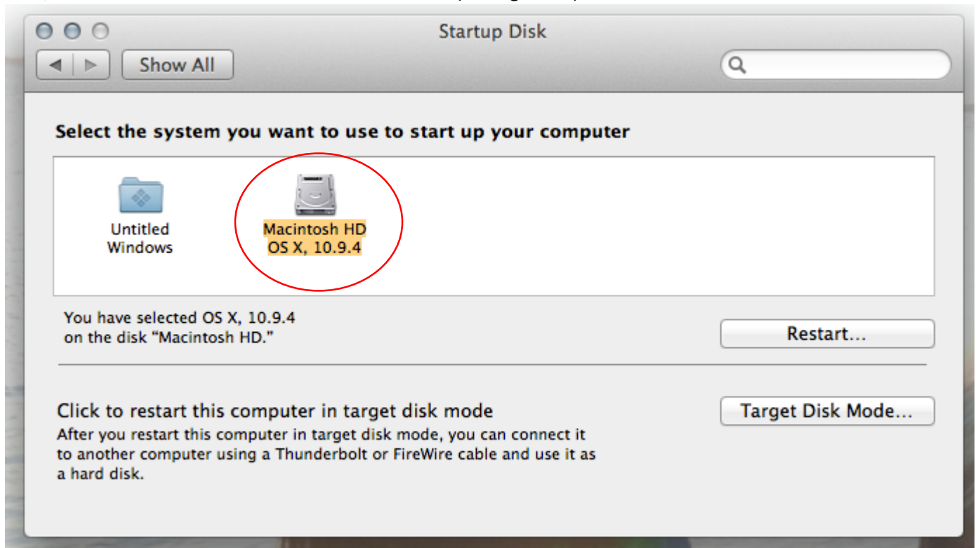
Figure 18 - For this example, Mac OS X is set up to start automatically
